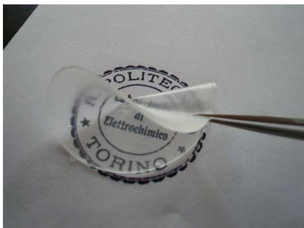
Fig. 1 Appearance of the BMPE gel-polymer membrane obtained by copolymerising the monomers BEMA and PEGMA via UV irradiation with the in situ addition of the 1:1 w/w EC-DEC solution
